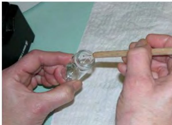
Figure 2-4-17 Golden Nematode Cyst Placement in Vial
