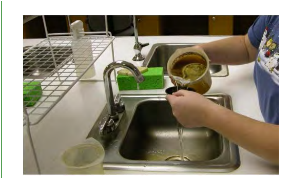
Figure 2-4-14 Pouring Sample from Beaker into Small #60 Sieve
