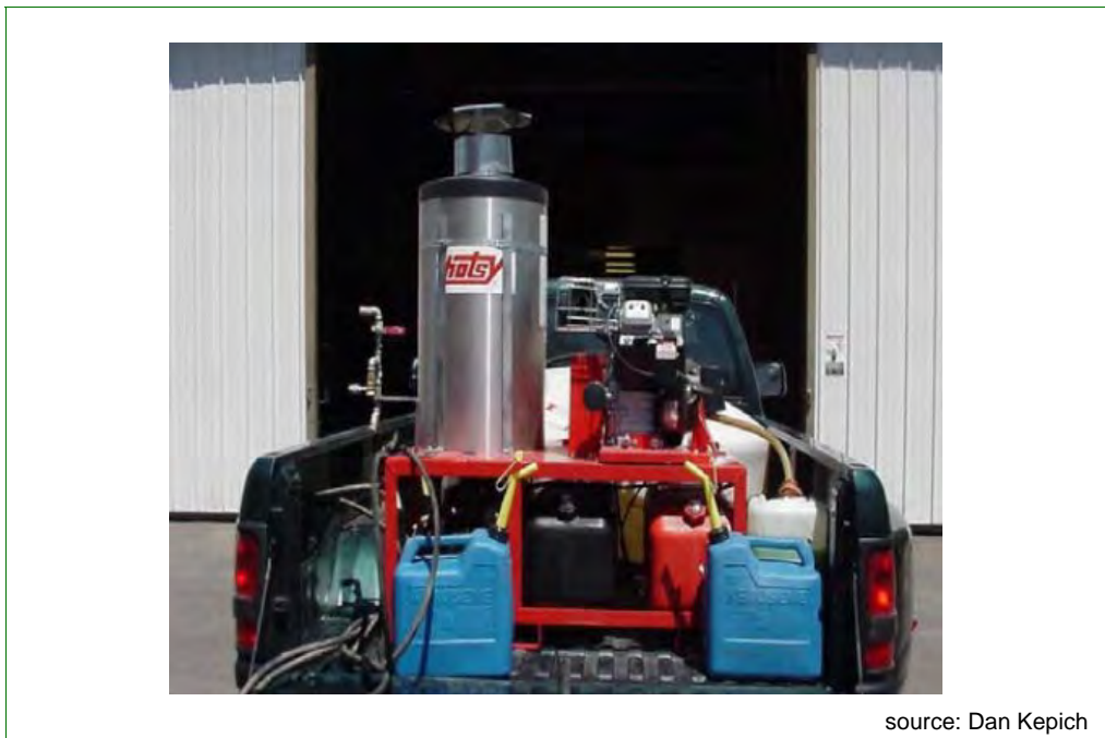
Figure 2-2-8 Pressure Washing Equipment and Supplies
