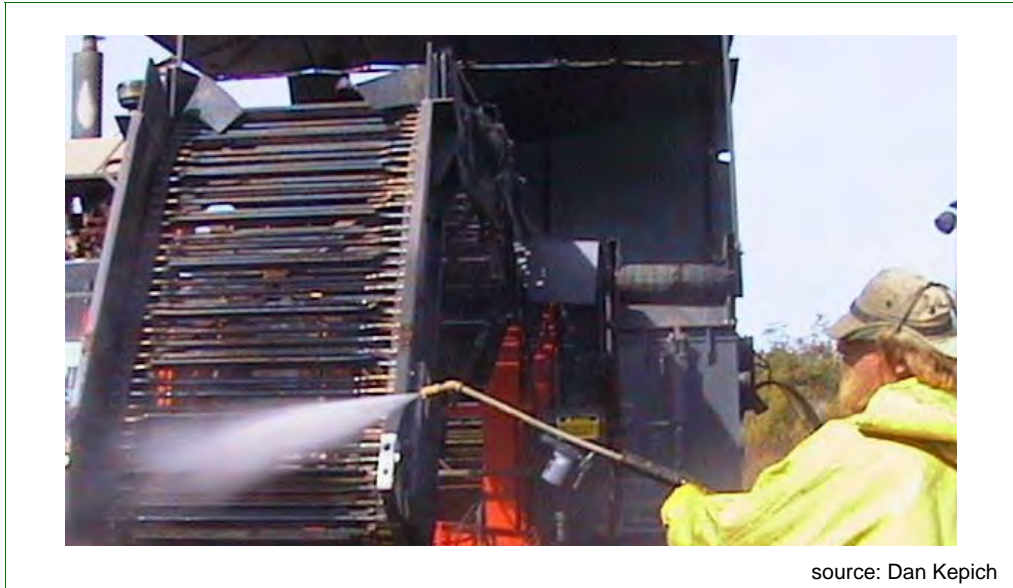
Figure 2-2-7 Pressure Washing With a Single Orifice Nozzle
