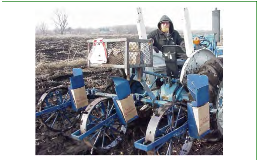
Figure 2-3-3 Three-Wheeled Mechanical Sampler
